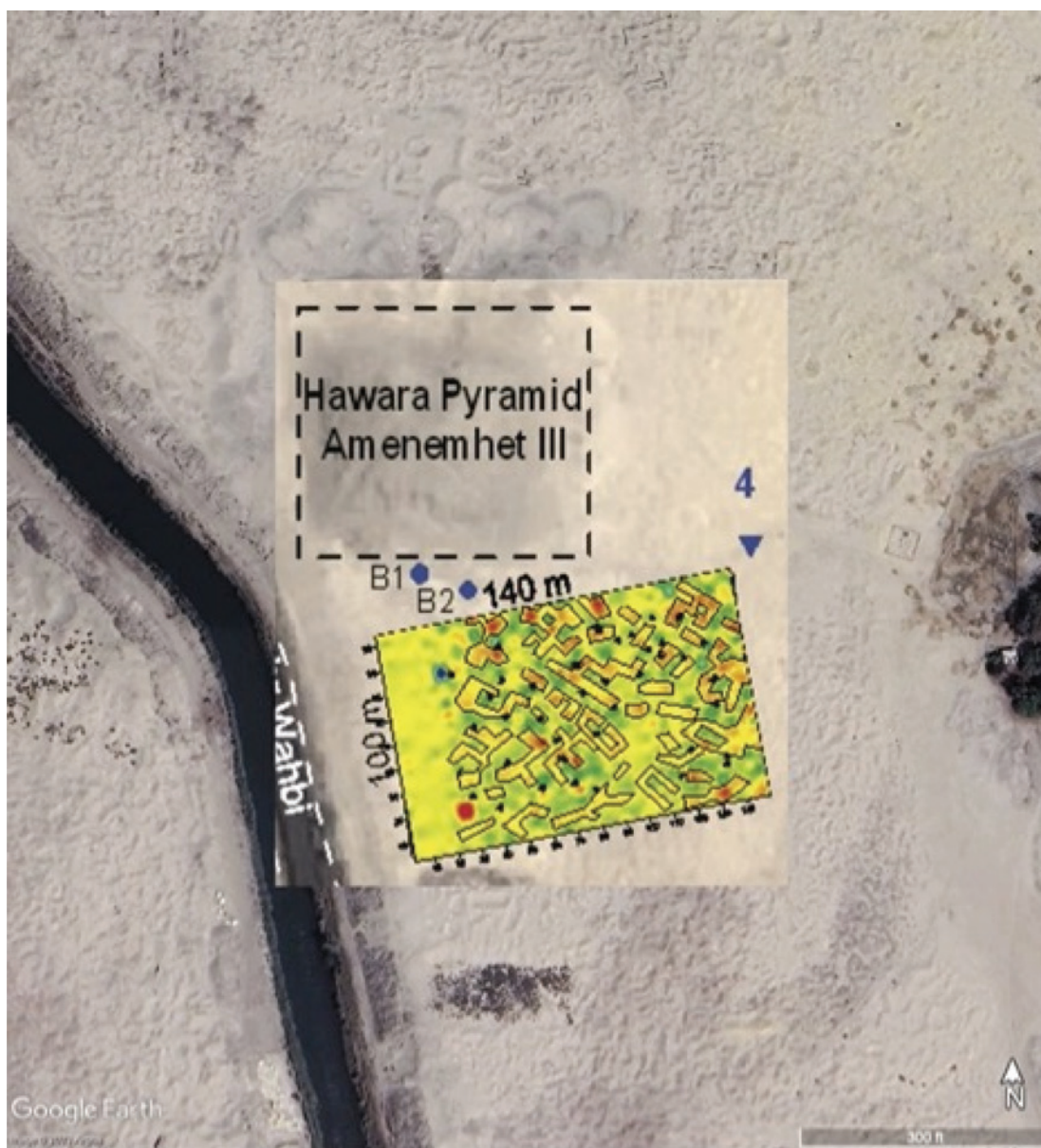
Figure 3. Map Derived from VLF-EM Data Registered to Google Earth. Red Colors are Conductive Zones (Archaeological Remains) and Green Colors are Resistive Zones (Host Soil).
