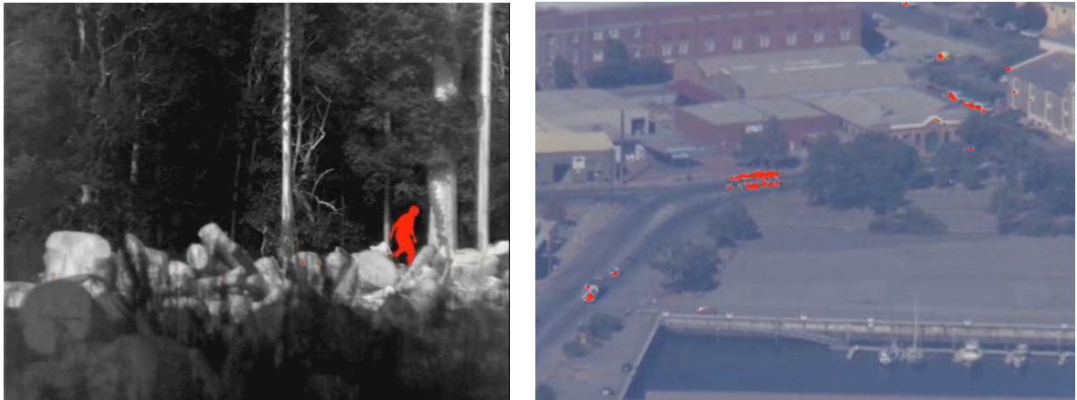
Figure 2 Moving object detection. Ground-based thermal IR video (left) and aerial video (right). (IR video courtesy NVL.)
