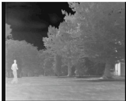
Two frames from TBC IR UGS video containing persons walking and moving background clutter. Pd = 1, compression ratio \sim 13,000:1
