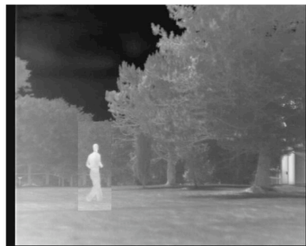
Two frames from TBC IR UGS video containing persons walking and moving background clutter. Pd = 1, compression ratio \sim 13,000:1
