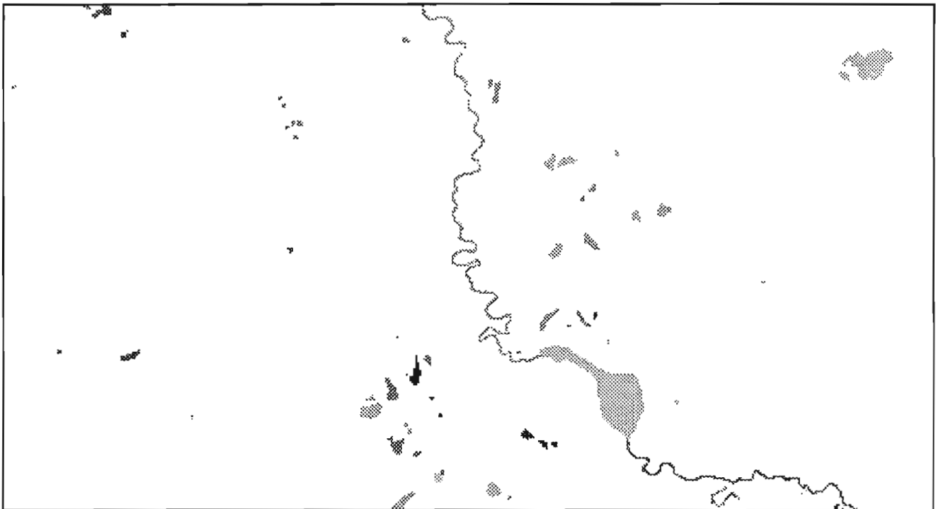
Fig. 10 Map of average water temperatures computed from thermal IR band. Relatively warm water is dark.
