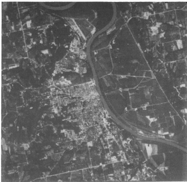
Fig. 2 Landsat TM image with bands 2, 3, and 5 in blue, green, and red.
