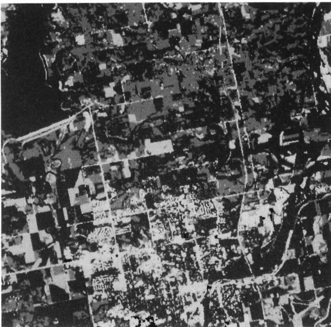
Fig 7 Soil-like materials: concrete and silt (white), plowed fields (dark-grey), other kinds of soil-like materials (dark-grey)
